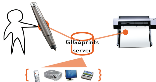
Figure 1. The Interactive Gigapixel Prints ensemble: wide-format inkjet printers, digital pens, and digital displays. This ensemble supports ambient awareness, visual context, and collaboration.
