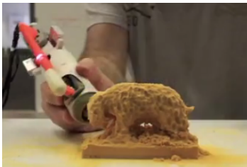
Figure 5: FreeD is an augmented sculpting tool that guides user movement.
